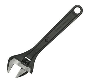
Features & Benefits ~ Forged chrome vanadium for strength & durability ~ Extra capacity jaws ~ up to 26% wider than standard patterns ~ Precision ground, fully polished jaws for secure nut engagement ~ Metric graduations for accurate jaw pre-setting ~ Capacity: 38 mm ~ Overall length: 300 mm
